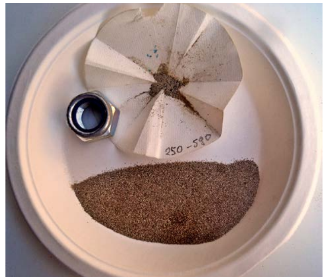
Fig. 7. Sandy clay from the Argille di Fangario formation (see text) - Sandy fraction, 590 \mu - 250 \mu interval, visual proportion of sinking and non-sinking (on filter paper) residue
