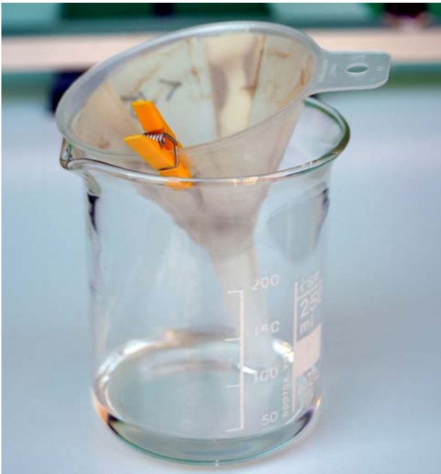
Fig. 6. Density separation with Perchloroethylene – recovering the non-sinking (floating + suspended) portion by filtering
