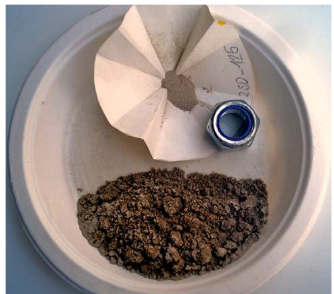
Fig. 8. Sandy clay from the Argille di Fangario formation (see text) - Sandy fraction, 250 \mu - 125 \mu interval, visual proportion of sinking and non-sinking (on filter paper) residue
